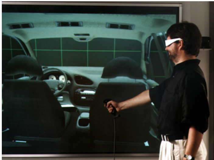
Powerwall with back projection
